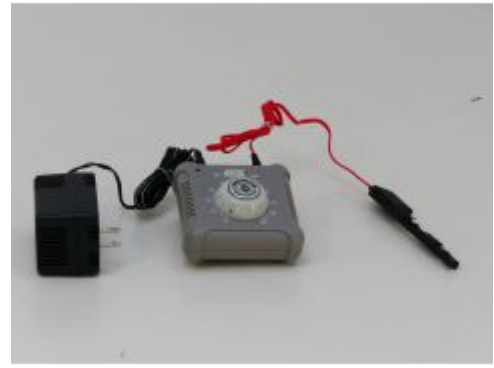
Bachmann Powerpack120V (Trafo, Rijregelaar, Snoer en Railverbinding)
