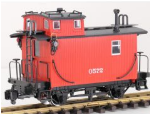
LGB 43653 Bobber Caboose No.0572, Klauwkoppelingen, Metallrader, Kugellager, Stromabnahme
